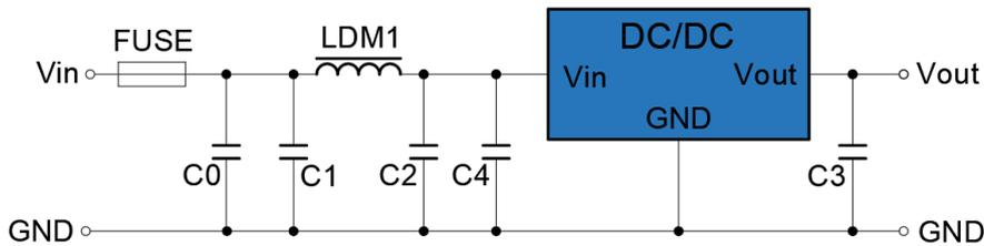
Figure 2. Recommended circuit diagram
